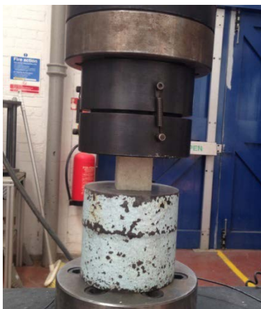
Figure 3. a) Compression test setup, b) tensile test setup of mortars.
