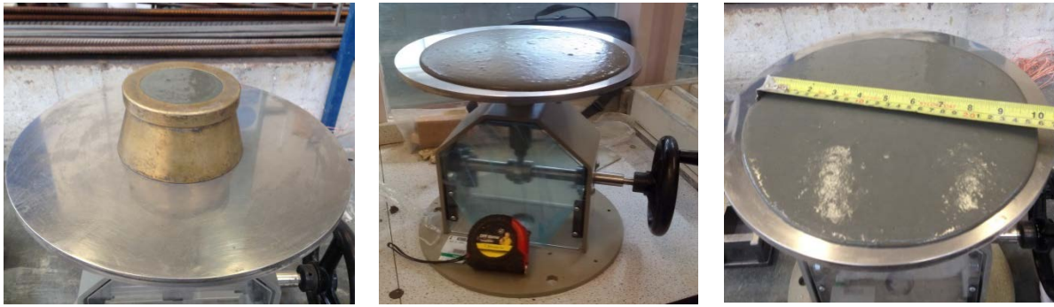
Figure 2. Flow table test setup of high strength fresh mortar.
