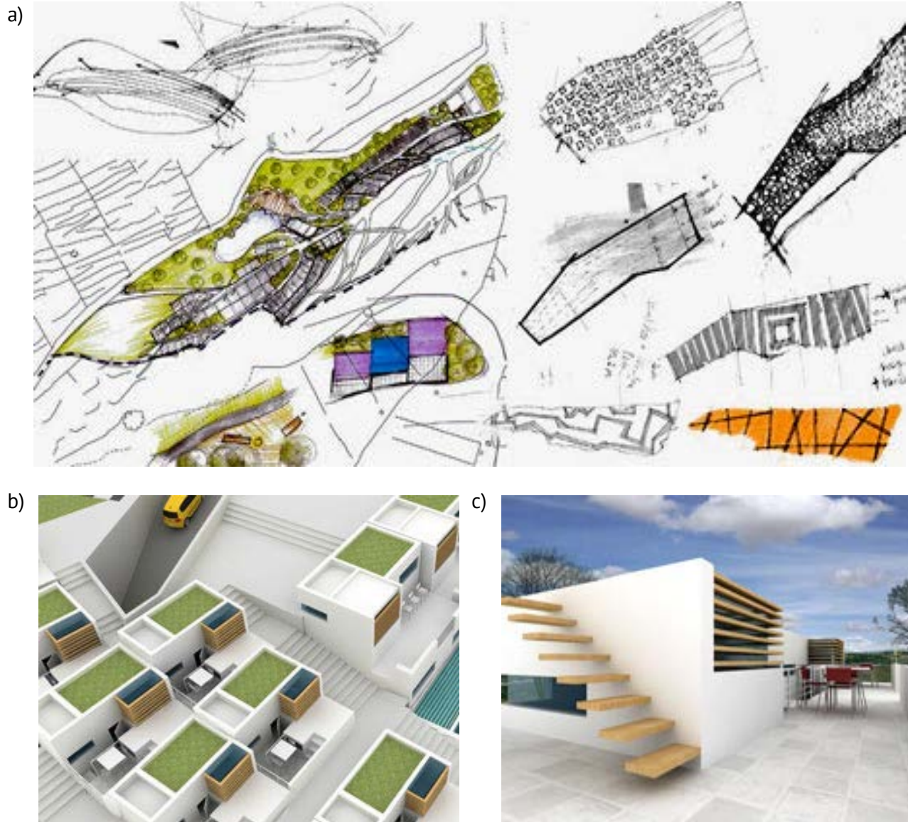
Figure 5. Upgrading of caravan and bungalow site in Malta (online version is in colour): a) concept sketches; b) computer generated 3-image of proposed development of the site; c) typical outdoor space to proposed units [5].
